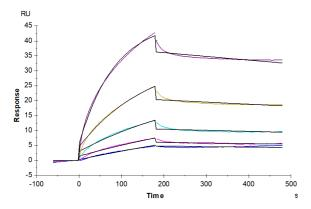
Human CD20 Nanodisc, His Tag captured on CM5 Chip via anti-his antibody can bind Rituximab, hFc Tag with an affinity constant of 3.09 nM as determined in SPR assay (Biacore T200).
